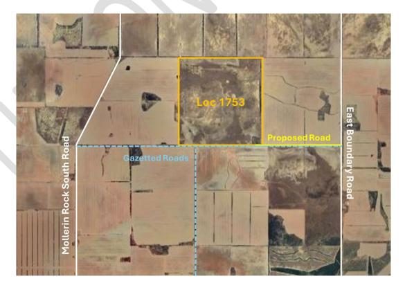
The most efficient provision of access to the block (Ninghan Loc 1753) both in distance and reduced vegetation clearance requirements is via the 1.8km road reserve to the property from East Boundary as depicted in yellow in the previous diagram.
